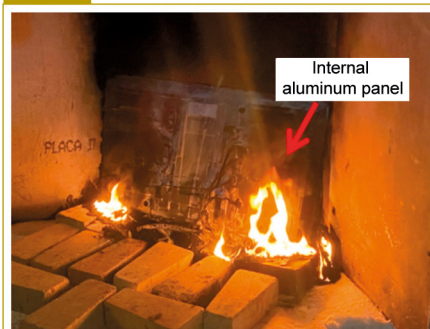
Picture 17 End of the real fire simulation test for the Brazilian TV
