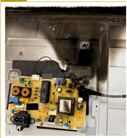
Picture 21 Internal damage to the American TV
