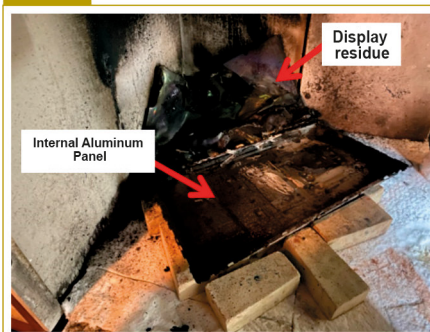
Picture 17 End of the real fire simulation test for the Brazilian TV
