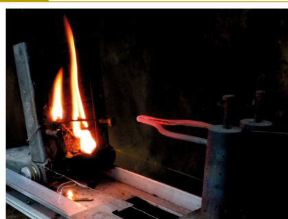
Picture 7 Brazilian TV casing: burning after the glow wire was removed and flare particles drop
