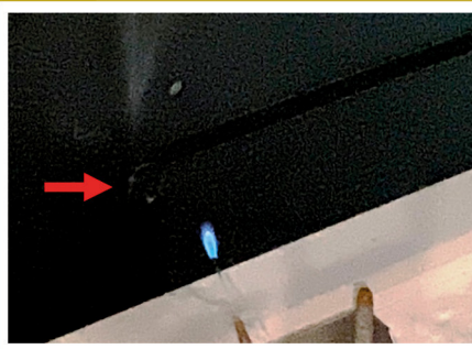
Picture 10 The American TV casing was not burned
