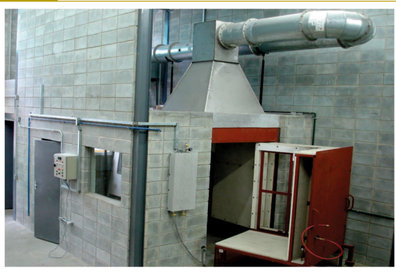
Picture 11 SBI equipment – Single Burning Item where the real fire simulations were performed for the Brazilian and American TVs
